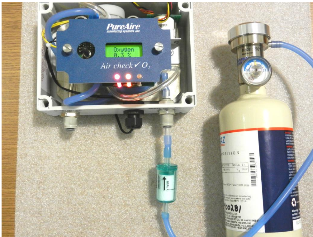
O 2 monitor Connected to gas cylinder
