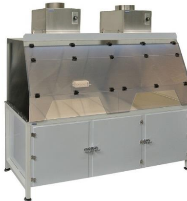
Stainless Steel Exhaust Hood with Chemical storage base cabinet and Built-in Blower and HEPA filter module. Clear Static dissipative PVC front tilt-up Sash
