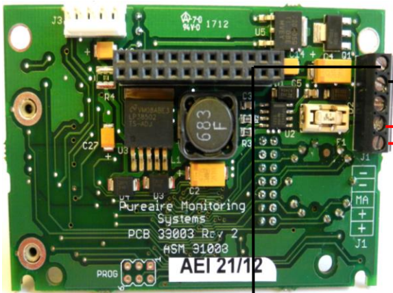
Oxygen Main Power Board
